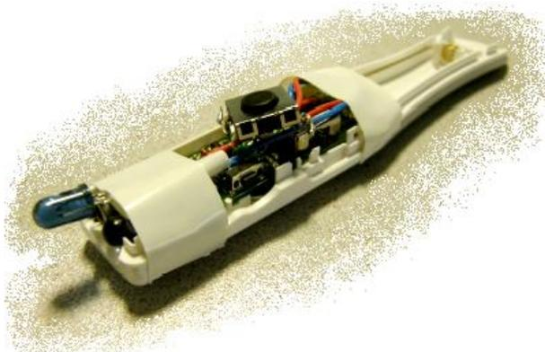
Figure 2 First 2D prototype: pen device version 1
