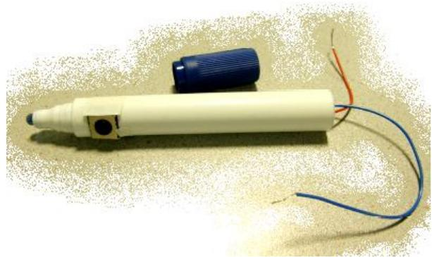
Figure 3 First 2D prototype: pen device version 2
