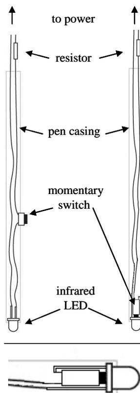
**Figure 5** From 2D handling prototype 1 to prototype 2 and zoom on the momentary switch linked to pen pressure
